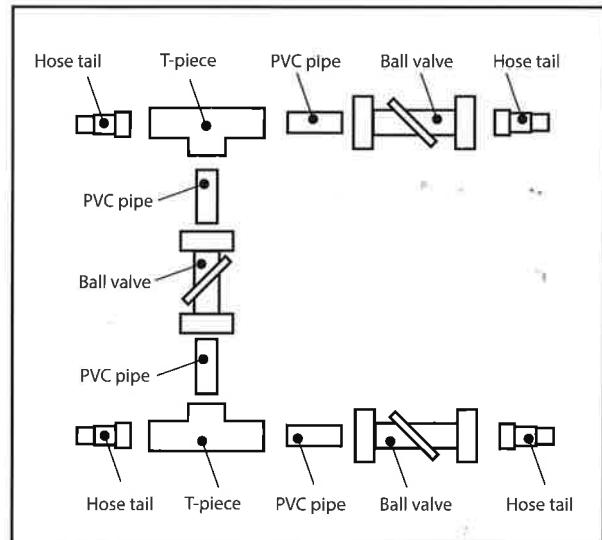
3. Connect the hoses of your pump/filter, heat pump and pool according to the instructions below.
