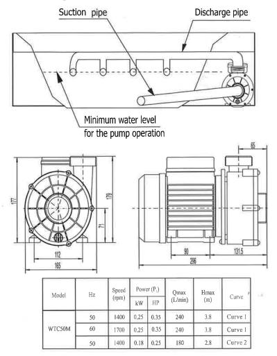
V/Hz esp: See pump nameplate. liquid temperature:  $4^{\circ}$ C  $\sim 50^{\circ}$ C Storage temperature:  $-10^{\circ}$ C  $\sim +50^{\circ}$ C. Relative Air Humidity:  $95^{\circ}$ Max.
